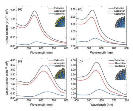
Fig. 2 Numerical simulations of extinction, absorption and scattering cross sections for (a) 15 nm diameter Au nanoparticles on  $SiO_2$  and (b-d)  $SiO_2$ -Au-Pt heterostructures with (b) a 0.5 nm thickness of Pt shell, (c) a 2 nm radius of Pt seeds and (d) a 0.5 nm Pt shell and 2 nm radius Pt seeds. Au nanoparticle size is the same for all simulations.
