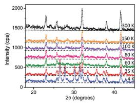
Fig. 7 Neutron diffraction data collected for Ca<sub>2</sub>Mn<sub>3</sub>O<sub>8</sub> showing the temperature dependence of the deviations/Warren-like behaviour of the background. Note the dotted line is a guide for the eve
