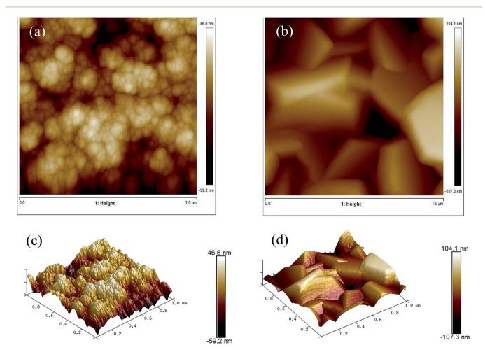
Fig. 7 AFM images of (a) undoped ZnO and (b) 10 mol% FeCl<sub>3</sub> doped ZnO and 3D images of the same area (c) and (d).
