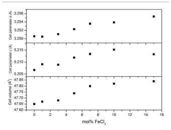
Fig. 5 Variation of cell parameters a, c and cell volume of the films with a change of mol% FeCl<sub>3</sub> added to the precursor solution. The increase of cell parameters confirms the incorporation of Cl into the ZnO lattice.
