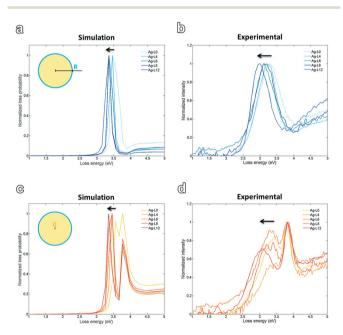
Fig. 5 Simulated spectra with impact parameter R (a) and 0 (c). Experimentally obtained EELS spectra show a similar trend for both impact parameters (b, d).
