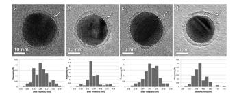
Fig. 2 BF-TEM images of (a) Aq-L4, (b) Aq-L6, (c) Aq-L8 and (d) Aq-L12 and corresponding distribution of the shell thicknesses.
