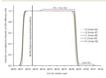
Fig. 7 Mass peak scan profile of a 250 ppb Ti run solution (0.3 M HNO<sub>3</sub> + 0.001 M HF) showing the alignment of individual Ti cups and a sufficiently flat low-mass shoulder plateau of >15 millimass units between peak edges and interference from  $^{36}\mathrm{Ar^{14}N^{+}}$  on  $^{50}\mathrm{Ti}$  in highresolution mode. The typical measurement position at X.926 is positioned in the middle of this plateau.
