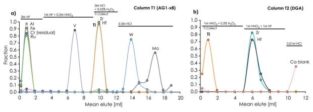
Fig. 4 Ion chromatographic elution profiles of elements separated on (a) the anion exchanger (600  $\mu$ l AG1-x8 200–400 mesh) column T1 (ID = 3.5 mm, L = 62 mm), which separates Ti (together with Zr and Hf) from Al, Fe, Ru, V, W and Mo, and (b) the 3<sup>rd</sup> Ti purification column (T2, ID = 3.5 mm, L = 27 mm) packed with 250  $\mu$ l of DGA-N 50–100  $\mu$ m resin.
