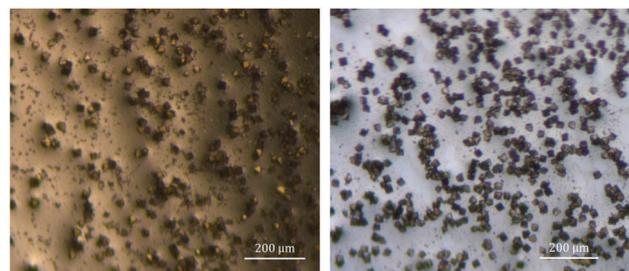
Fig. 1 Optical micrographs of single crystals of the {Np<sub>38</sub>} compounds synthesised from THF (1, left) and isopropanol (2, right).
