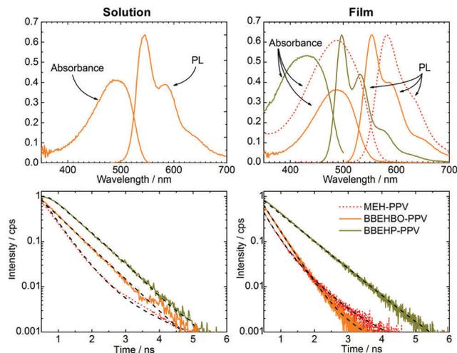
Fig. 1 Top: Absorption and PL spectra of BBEHBO-PPV in solution at 0.025 mg ml<sup>-1</sup> (top left) and as a film (top right). The absorption and PL spectra of MEH-PPV and BBEHP-PPV as films are also shown top right. Bottom: Photoluminescence lifetime measurements in solution (bottom left) and film (bottom right) for BBEHP-PPV, MEH-PPV and BBEHBO-PPV.
