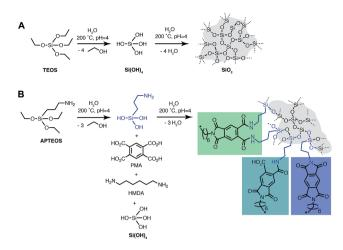
Fig. 4 Reaction equation of  $SiO_2$  and  $PI6/SiO_2$  co-condensation. (A) Hydrothermal hydrolysis and condensation sequence from TEOS to  $SiO_2$ . (B) Co-condensation of PI6 and  $SiO_2$  in the presence of the compatibilizer APTES; possible linkages (1,2-diamide, amic acid; and imide) are shown.
