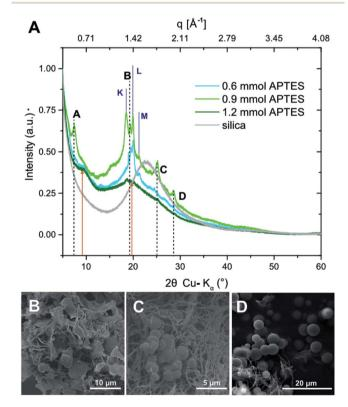
Fig. 6 PI6/SiO<sub>2</sub> prepared from PMA, HMDA, APTES and TEOS. (A) Diffractograms of the hybrids prepared at different  $n_{APTES}$ , and diffractogram of hydrothermally synthesized  $SiO_2$  for comparison (gray). (B)–(D) SEM images of the corresponding hybrids at  $n_{APTES} = 0.6$  mmol (B),  $n_{APTES} = 0.9$  mmol, and  $n_{APTES} = 1.2$  mmol.
