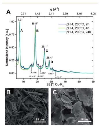
Fig. 3 Crystallinity of hydrothermally prepared PI6. (A) PXRD pattern of PI6 prepared at 200 °C and pH =4 at  $t_R=2$  h (dark blue); 4 h (green) and 24 h (turquoise). Reflections are labelled (A)–(J) with annotated scattering angles  $2\theta$  (Cu-K $_{\!\alpha}$ ). (B) SEM image of PI6 synthesized at 200 °C and pH =4 for 24 h. (C) SEM image of PI6 synthesized at 200 °C and pH =1 for 24 h.
