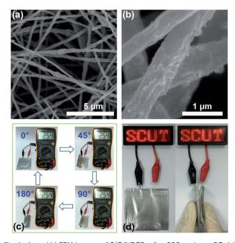
Fig. 4 (a and b) SEM images of S/G/NPCFs after 500 cycles at 5C; (c) the open-circuit voltage of a flexible battery using the S/G/NPCF electrode as the cathode at different bending angles  $(0-180^{\circ})$ ; (d) photographs of the LED device lit by the flexible battery during folding.
