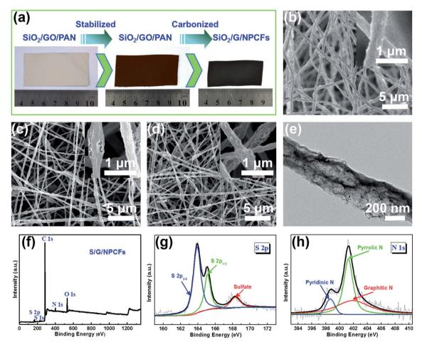
Fig. 1 (a) The photographs of the calcination process of the as-prepared film; (b) typical SEM images of GO/SiO<sub>2</sub>/PAN, (c) G/NPCFs and (d) S/G/NPCFs; (e) TEM image of S/G/NPCFs. (f) XPS spectrum of S/G/NPCFs; high resolution spectra of (g) S 2p and (h) N 1s of S/G/NPCFs.
