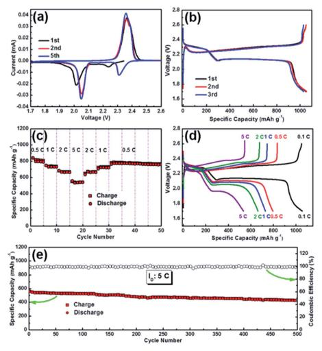
Fig. 3 (a) CV curves for selected cycles of the S/G/NPCF electrode tested at a scan rate of 0.2 mV s<sup>-1</sup> in the potential range from 1.7 to 2.6 V; (b) typical discharge–charge curves of S/G/NPCFs at 0.1C for the first three cycles; (c) rate capability of the S/G/NPCFs electrode recorded at current rates of 0.5C, 1C, 2C, and 5C; (d) typical discharge–charge curves of S/G/NPCFs at different current densities; (e) long-term cycling performance of S/G/NPCFs at 5C.
