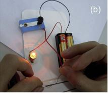
Fig. 28 (a) Flexible RFID antenna printed with nano-Cu ink with on photopaper using a roller ball pen and (b) a conductive test of nano-Cu ink patterns using an ordinary lamp. [Reprinted with permission from ref. 266 Copyright © Elsevier.]
