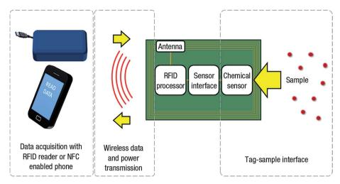
Fig. 3 Schematic illustration of an RFID-based tag chemical sensor platform and its operating principle. [Reprinted with permission from ref. 103. Copyright © Elsevier.]
