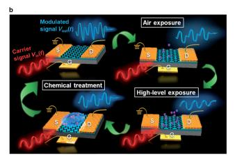
Fig. 13 (a) The nodal architecture of an Internet of nano things using nanomaterial-based sensing modulators. (b) Conceptual illustration of the chemical-sensitive graphene based modulator. [Reprinted with permission from ref. 193 Copyright © Macmillan Publishers Limited/Springer Nature.]
