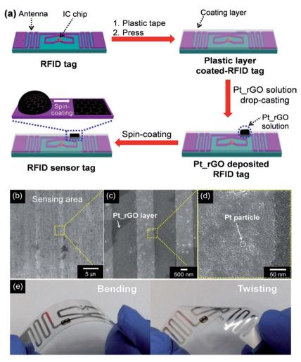
Fig. 10 (a) Fabricating process of PtNPs/rGO hybrid-based flexible RFID sensor tag. Field-effect scanning electron microscopy (FE-SEM) images of the PtNPs/rGO hybrid sensing area at (b) low-, (c) middle-, and (d) high-resolution. (e) Photographs showing flexibility of RFID sensor tag under bending and twisting conditions. [Reprinted with permission from ref. 187 Copyright © American Chemical Society.]
