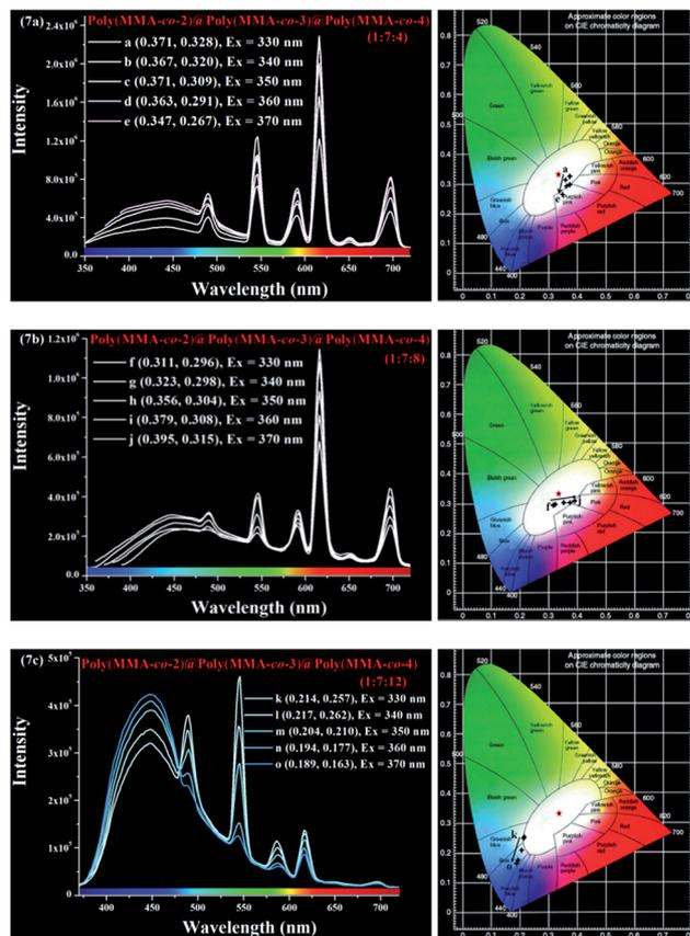
Fig. 7 Emission spectra (left) and corresponding CIE coordinates (right) of polymers' blends **Poly(MMA-co-2)**@**Poly(MMA-co-2)**@**Poly(MMA-co-2)** with different doping mass ratios (1 : 7 : 4, 1 : 7 : 8 and 1 : 7 : 12) in the solid state at room temperature upon excitation: (7a) 1 : 7 : 4; (7b) 1 : 7 : 8; (7c) 1 : 7 : 12.
