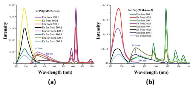
Fig. 6 Emission and excitation spectra ( $\lambda_{\text{ex}} = 341 \text{ nm}$ ) of homo- $\text{Ln}^{3+}$ -grafted polymers with different feed molar ratios (100 : 1, 200 : 1, 400 : 1 and 600 : 1) in the solid state at room temperature; (6a) for Poly(MMA-co-2); (6b) for Poly(MMA-co-3).
