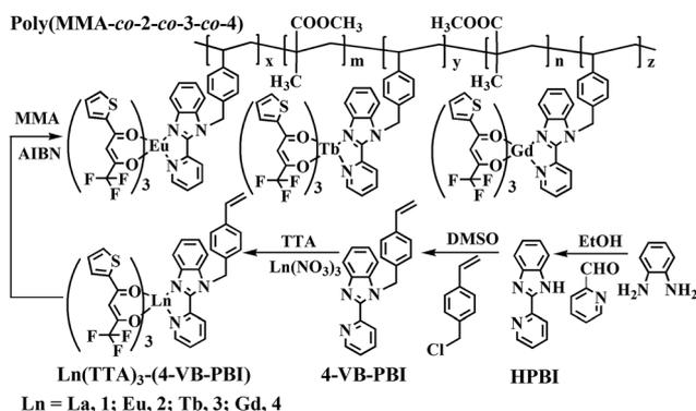
**Scheme 1** Reaction scheme for the synthesis of the vinyl-functionalized complex monomers **1–4** and  $\text{Eu}^{3+}$ - $\text{Tb}^{3+}$ - $\text{Gd}^{3+}$ -grafted polymer Poly(MMA-co-2-co-3-co-4).
