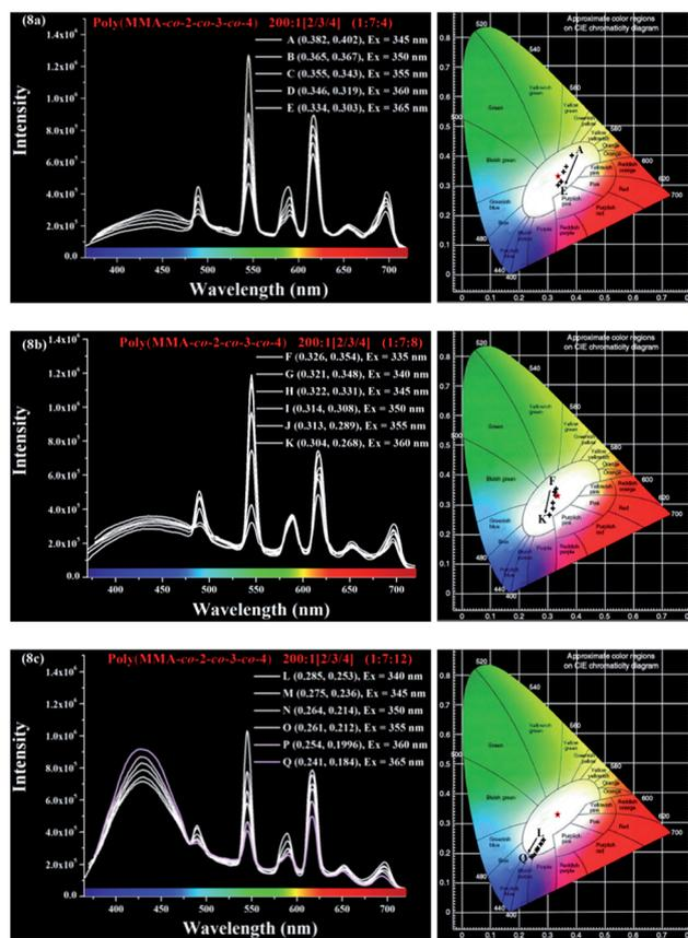
Fig. 8 Emission spectra (left) and corresponding CIE coordinates (right) of Eu<sup>3+</sup>-Tb<sup>3+</sup>-Gd<sup>3+</sup>-grafted polymers Poly(MMA-co-2-co-3-co-4) in the solid state at room temperature upon excitation: (8a) 200 : 1(2/3/4) = 1 : 7 : 4; (8b) 200 : 1(2/3/4) = 1 : 7 : 8; (8c) 200 : 1(2/3/4) = 1 : 7 : 12.
