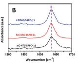
Fig. 6 IR spectra of pyridine (A) and 2,6-dimethylpyridine (B) adsorption for (a) C-HTC-SAPO-11, (b) C-SAC-SAPO-11 and (c) SISAC-SAPO-11 samples at 423 K.
