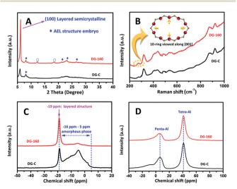
Fig. 1  $\,$  XRD patterns (A), Raman spectra (B),  $^{31}P$  (C) and  $^{27}Al$  MAS NMR spectra (D) of synthesized DG-C and DG-160.
