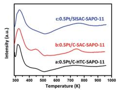
Fig. 7 H<sub>2</sub>-TPR profiles of (a) C-HTC-SAPO-11, (b) C-SAC-SAPO-11 and (c) SISAC-SAPO-11.
