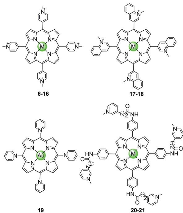
Fig. 3 Metal-TMPyP4 complexes and derivatives reported as G4-ligands. The metal centres in complexes **6–16** are Ni(II), Mn(III), Mn(V)=O, Mg(II), Cu(II), Zn(II), Pd(II), Pt(II), Fe(III), Co(II), In(III), in **17–18** Cu(II) and Zn(II), and in **20–21** Mn(III) and Ni(II), respectively.<sup>44–54</sup>
