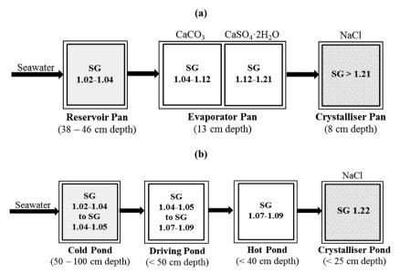
Fig. 3 Schematic illustration of salt production in (a) Goa, India<sup>56</sup> and (b) Maristella salt works at the Western Sicilian Coast.<sup>58</sup> (SG represents the specific gravity calculated from °Bé using the formula SG = 1.45/(1.45 - °Bé)).
