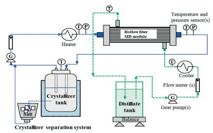
Fig. 6 Schematic flow sheet of a typical MDC (redrawn from Curcio et al. 71).
