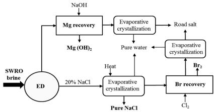
Fig. 5 Schematic illustration of SWRO brine treatment with ED and recovery of NaCl, Br<sub>2</sub> and Mq(OH)<sub>2</sub>.<sup>23</sup>
