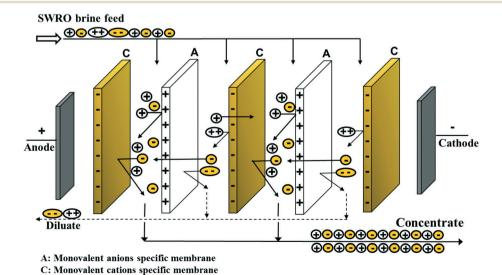
Fig. 4 Schematic illustration of the electrodialysis process used to concentrate SWRO brine prior to salt production by evaporation.
