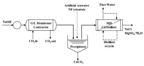
Fig. 7 Schematic flow sheet of a process of mining CaCO<sub>3</sub>, NaCl and MgSO<sub>4</sub>.7H<sub>2</sub>O from artificial seawater NF retentate using MDC (redrawn from Drioli et al.21).
