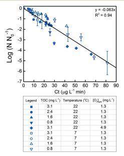
Fig. 1 Summary of L. pneumophila inactivation at 7 and 22 °C with various initial TOC loadings and initial ozone concentrations generated when the ozone generator was driven at 50 V ( $C_{gi} = 1.3 \text{ g m}^{-3}$ ) and 120 V ( $C_{qi}$  = 4.9 g m<sup>-3</sup>). Data plotted are average values and standard deviations of at least three replicates.
