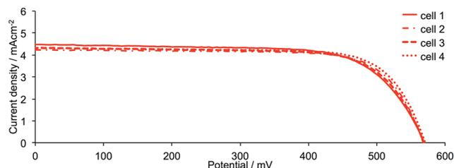
Fig. 5  $J$ - $V$  curves for sets of four DSCs containing the dye  $[\text{Cu}(2)(6)]^+$  measured on the day of cell assembly to confirm performance reproducibility. Analogous sets of data for DSCs containing the dyes  $[\text{Cu}(2)(3)]^+$ ,  $[\text{Cu}(2)(4)]^+$  and  $[\text{Cu}(2)(5)]^+$  are shown in Fig. S1.†
