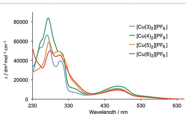
Fig. 2 Solution (CH<sub>2</sub>Cl<sub>2</sub>) absorption spectra of complexes [Cu(L<sub>ancillary</sub>)<sub>2</sub>][PF<sub>6</sub>] with L<sub>ancillary</sub> = **3–6** (5 × 10<sup>-5</sup> mol dm<sup>-3</sup>).
