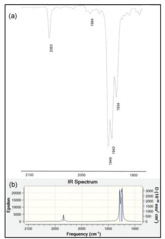
Fig. 6 (a) Experimental solution IR spectrum in the carbonyl stretching region of 10 measured dilute in hexane. (b) Computed gas-phase IR spectrum at the B3PW91/LANDL2DZ level of theory (data in Table 3).
