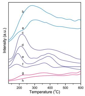
Fig. 4 NH<sub>3</sub>-TPD curves of the fresh aluminosilicate catalysts: (a) SA@0.03, (b) SA@1.79, (c) ZSM-5@30, (d) ZSM-5@64, (e) ZSM-5@106, (f) ZSM-5@260, (g) Al-SBA-15@102 and (h) Al-SBA-15@190
