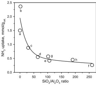
Fig. 5 Evolution of the total acidity on the fresh aluminosilicate catalysts measured by NH<sub>3</sub>-TPD as a function of the SiO<sub>2</sub>/Al<sub>2</sub>O<sub>3</sub> ratio: (a) SA@0.03, (b) SA@1.79, (c) ZSM-5@30, (d) ZSM-5@64, (e) ZSM-5@106, (f) ZSM-5@260, (g) Al-SBA-15@102 and (h) Al-SBA-15@190.
