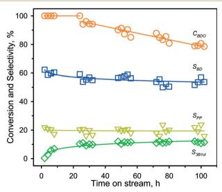
Fig. 2 Catalytic stability over ZSM-5@260 at 300 °C. Reaction conditions: T, 300 °C; ambient pressure, catalyst loading, 200 mg; liquid flowrate, 2.8 mL h<sup>-1</sup>; carrier gas flowrate, 60 mL (STP) min<sup>-1</sup>. Nomenclature:  $C_{BDO}$ , 1,3-BDO conversion;  $S_{BD}$ , selectivity to BD;  $S_{PP}$ , selectivity to PP;  $S_{3B1ol}$ , selectivity to 3-buten-1-ol.
