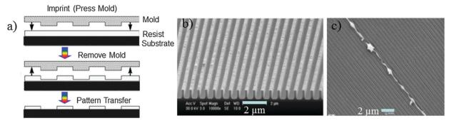
Fig. 4 (a) Scheme of nanoimprinting. (b) NIL results using a 250 nm line width PDMS-b-PS grating. (c) 400 nm width and 800 nm pitch. SEM images show that the axons grow on the ridge edges, and not in the grooves. Reprinted with permission. 54,58 Copyright 2007 and 2004, Wiley-VCH.
