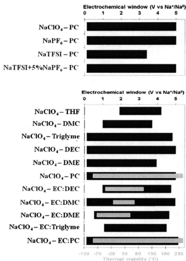
Fig. 15 Electrochemical potential window stability of various salts with PC and  $\text{NaClO}_4$  in various solvents. Reproduced with permission<sup>150</sup> © 2012, RSC Publishing.
