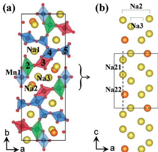
Fig. 5 (a) Crystal structure of  $\text{Na}_{0.44}\text{MnO}_2$  showing Mn and Na binding sites, and (b) the S shaped tunnel configuration along  $c$ -axis with different sodium positions Na21 and Na22 in  $\text{Na}_{0.44}\text{MnO}_2$ . Reproduced with permission<sup>55</sup> © 2012, ACS Publications.
