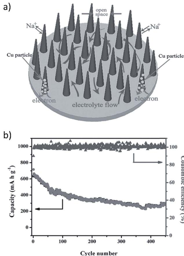
Fig. 14 (a) Binder free CuO nanowire array (CNA) electrode, and (b) cycling performance of the binder free CNA (current density 200 mA g<sup>-1</sup>). Reproduced with permission<sup>148</sup> © 2014, WILEY-VCH Verlag GmbH & Co.
