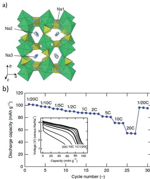
Fig. 8 (a) Na<sub>2</sub>Fe<sub>2</sub>(SO<sub>4</sub>)<sub>3</sub> structure projected along the *c* axis, and (b) capacity retention upon cycling up to 30 cycles under various rate of C/20 (2 Na in 20 h) to 20 C. Reproduced with permission<sup>80</sup> © 2014, Nature Publishing Group.
