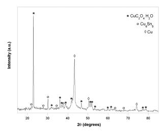
Fig. 4 WA-XRD spectrum and peaks assignment for Cu(C<sub>2</sub>O<sub>4</sub>)·H<sub>2</sub>O precipitate obtained from the leaching of 10 g of test specimen by citric acid 3M at room temperature and H<sub>2</sub>O<sub>2</sub> 35% addition.
