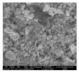
Fig. 5 SEM micrograph of copper recovered by cementation with Zn. Average particles size =  $\sim$ 500 nm.
