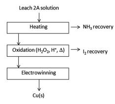
Fig. 7 Schematic diagram of Cu(s) electrochemical recovery from a Leach 2A solution. Reagent recovery/valorisation.
