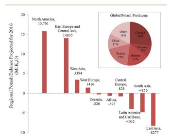
Fig. 1 Projection of the regional potash balance of import vs. export according to the FAO for 2016 (ref. 3) in million metric tonnes of K2O equivalent. Inset shows the current national distribution of potash producers.
