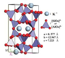
Fig. 2 Idealized crystalline structure of microcline: the red spheres represent oxygen atoms; silicon and aluminum atoms are within the [SiO<sub>4</sub>]<sup>4-</sup> and  $[AlO_4]^{5-}$  tetrahedra, and the potassium charge-balancing cations are the blue spheres.
