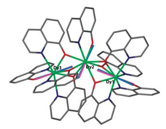
Fig. 7 Magnetic anisotropy axes for  $[Dy_3(8-quinolinolate)_9]$ . Blue rods are from ab initio calculations, while pink rods are from electrostatic calculations. Hydrogen atoms are omitted for clarity. Reprinted with permission from ref. 23. Copyright 2014 American Chemical Society.
