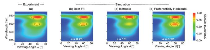
Fig. 2 TM-polarized part of the spectral radiant intensity for the OLED stack with  $Ir(dhfpy)_2(acac)$ . (a) Experimental data, (b) simulated data for the best fit (a = 0.25), (c) simulation assuming isotropic orientation (a = 1/3) and (d) simulation assuming slightly stronger horizontal orientation (a = 0.25). All intensities are normalized to the maximum intensity and are plotted on a linear false-color scale.
