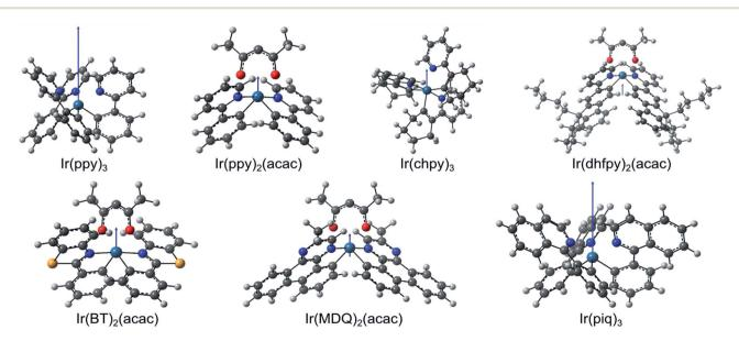
Fig. 3 DFT optimized molecular structure, calculated relative magnitude and orientation of permanent dipole moment  $\mu$  (blue arrows) for all phosphorescent emitter molecules investigated here. All dipole moments originate at the center of charge.
