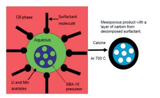
Fig. 1 A schematic diagram showing the formation of mesoporous manganese deficient lithium manganese silicate from SBA-15 using emulsion synthesis.
