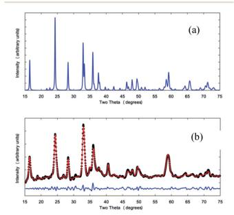
Fig. 4 (a) A simulated X-ray diffraction pattern of  $\rm Li_2MnSiO_4$  (b) Rietveld refinement results of structural models with the powder XRD pattern of the mesoporous Mn-deficient product phase. Black dots represent the experimental data, the model is the red line through the data and the blue line below is the difference between the model and the data.
