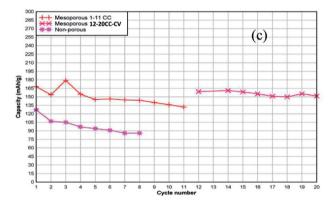
Fig. 5 Galvanostatic cycling curves of half-cells containing mesoporous cathodes (a) cycles 1-10 CC cycling (b) cycles 12-20 CC-CV cycling at room temperature and 20 mA  $\rm g^{-1}$  (c) capacity  $\it vs.$  cycle number.
