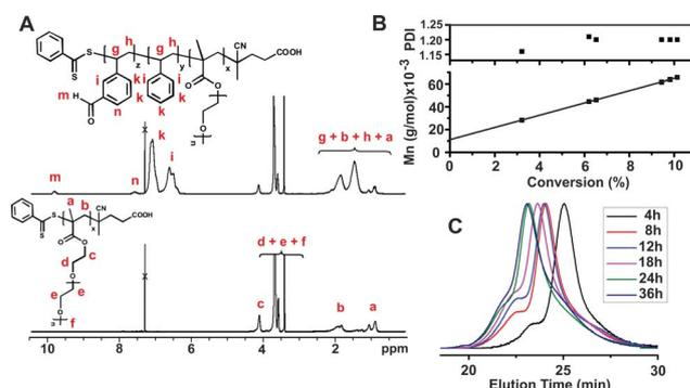
Fig. 1 (A) <sup>1</sup>H-NMR spectra of POEGMA and POEGMA-*b*-P(ST-*co*-VBA) polymers (recorded in CDCl<sub>3</sub>); (B) evolution of molecular weight and PDI versus monomer conversion; (C) evolution of GPC traces versus polymerization times.
