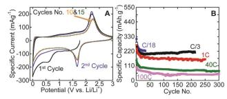
Fig. 3 Electrochemical performance of flash-oxidized  $Ti_3C_2T_x$  powders in LIBs (A) CVs at a rate of 0.2 mV s<sup>-1</sup>; (B) effect of cycling on Li capacity at various rates.
