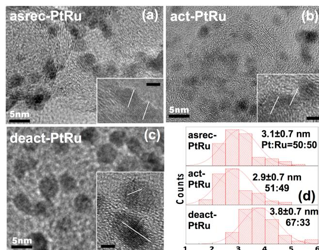
Fig. 4. The TEM images of the asrec-PtRu (a), act-PtRu (b), and (c) deact-PtRu. (d) shows the size distributions of the three samples (200 counts per sample) and their elemental ratios measured by EDS. The insets in (a) through (c) are high resolution TEM images with the white straight lines highlighting the atomic planes and crystallinity of the samples. The scale bars are 5 nm and 2 nm for the main images and the insets respectively.
