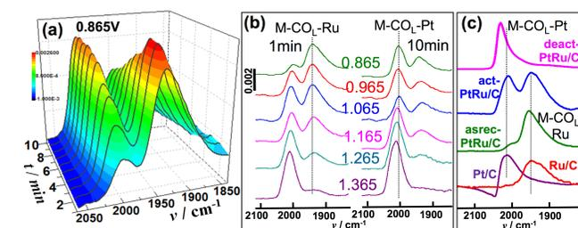
**Fig. 2.** In situ SEIRAS spectra of M-CO<sub>L</sub> on the J-M PtRu/C: (a) the time-dependent IR spectra of CO during SPS-1; (b) the IR spectra of M-CO<sub>L</sub> after the first (left) and tenth SP (right) as the SP value changes from 0.865 V to 1.365 V; (c) the IR spectra of M-CO<sub>L</sub> on asrec- (green), act- (blue), deact- (magenta) PtRu, Pt/C (brown), and Ru/C (red), respectively.
