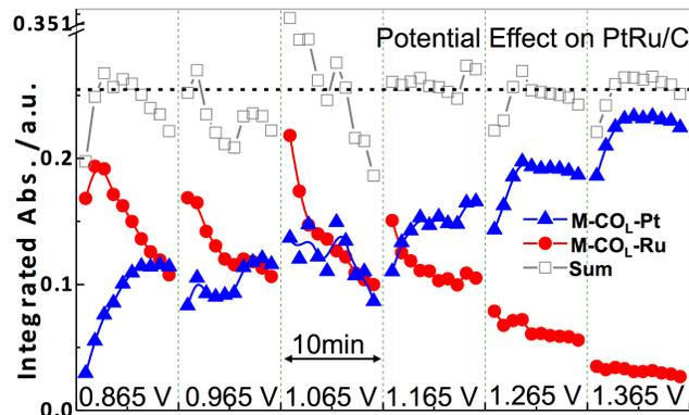
Fig. 3. The integrated IR band intensities of the M-CO<sub>L</sub>-Pt (blue triangles), -Ru (red circles), and sum of the both (open squares) as a function of time per a given SPS and of the SPS.
