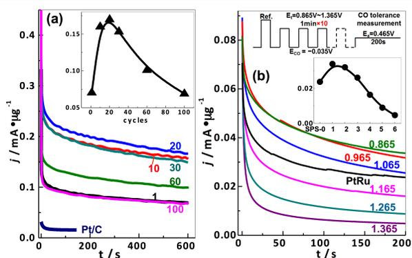
**Fig. 1.** CA curves of the J-M PtRu/C deposited on GC (glassy carbon) after multiple potential cycles together with that of the J-M Pt/C as a reference (a) and the SPSs on Au film (b). The inset in (a) shows the potential-cycle-dependent mass specific MOR activity at 0.495 V. The insets in (b) are the schematic of an SPS and the SPS-dependent mass specific MOR activity at 0.465 V respectively.
