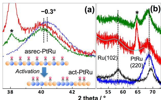
**Fig. 5.** The XRD patterns of the asrec-PtRu (blue), act-PtRu (red), and deact-PtRu (green). The black spectrum in (b) was from Ru/C, shown here as a reference. The stars indicate the peaks from the underlying Au thin film deposited on the Si prism for SEIRAS. The schematic inset in (a) illustrates the proposed activation process. Orange, blue, black and pink balls stand for the Pt, Ru, C and O atoms respectively.
