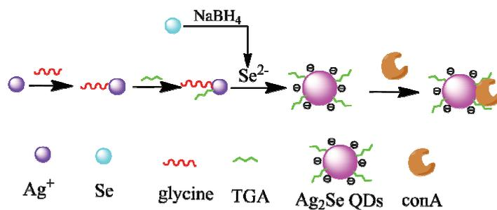
Schematic illustration for fabricating TGA and glycine modified  $\text{Ag}_2\text{Se}$  QDs for RRS detection of conA
