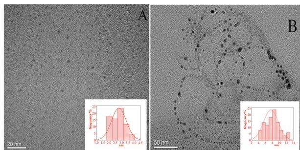
**Fig.1** (A) TEM image of Ag<sub>2</sub>Se QDs. (B) TEM image of Ag<sub>2</sub>Se QDs-conA complex.
