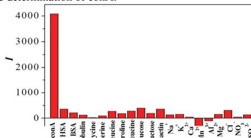
Fig. 8 Selectivity of Ag<sub>2</sub>Se QDs probe towards conA. Ag<sub>2</sub>Se QDs, 5×10<sup>-4</sup> mol/L; pH=6.0; SCBS buffer 300μL; conA 35 μg/mL. The concentrations of all samples were 5mmol/L.
