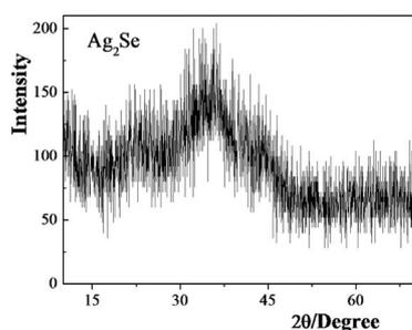
**Fig.2** XRD pattern of Ag<sub>2</sub>Se QDs.
