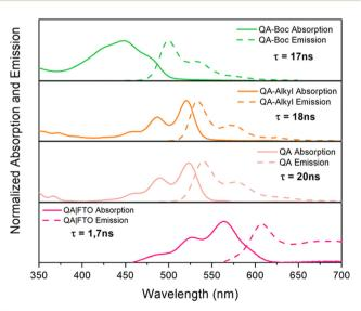
Fig. 1 Normalised absorption and emission properties of QA derivatives. QA-Boc, QA-alkyl and QA spectra are reported in DMSO solution; spectra of QA films prepared by vacuum sublimation over FTO are registered under air atmosphere. For the emission spectra, the major lifetime component is also indicated.
