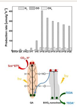
Fig. 8 Top panel: Production rates from CO<sub>2</sub> photoreduction (average over 10 h) on  $BiVO_4$ , QA, and  $QA/nBiVO_4$  for 10 h. n is the mass ratio between BiVO<sub>4</sub> and QA, impacting the photocatalytic performance. Bottom panel: Schematic representation of photochemical CO2 reduction on QA/BiVO<sub>4</sub> composites. Reproduced from ref. 50 with permission from Wiley Inc., copyright 2020.
