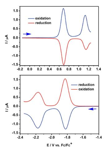
Fig. 2 Differential pulse voltammograms registered for N,N'-dioctyl QA (DOQA) in DCM. Reproduced from ref. 32 with permission from the Royal Society of Chemistry, copyright 2017.
