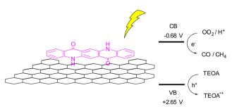
Fig. 7 Reduction of CO<sub>2</sub> over QA/rGO photocatalyst, and schematic representation of CO<sub>2</sub> reduction to CO and CH<sub>4</sub>, coupled with oxidation of triethanolamine (TEOA); the potential of the conduction and valence bands (CB and VB, respectively) are reported versus the reversible hydrogen electrode.49
