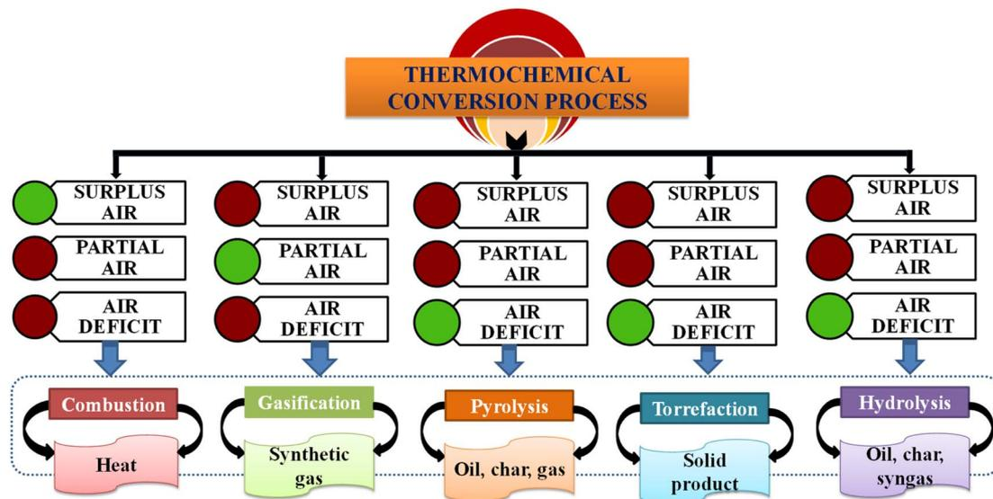
Fig. 3 Concept of thermochemical conversion processes of biomass.
