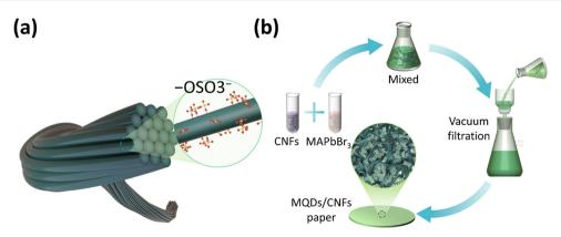
Fig. 1 (a) Illustration of sulfated CNFs. (b) Fabrication of MQDs/CNF papers via a vacuum filtration method
