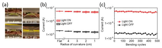
Fig. 6 (a) Photograph of the flexible MQDs@10/CNF paper photodetector under different bending conditions. (b)  $l_{on}$  and  $l_{off}$  of the MQDs@10/CNF photodetector measured with various bending curvature from flat, 4, 3, 2, to 1 cm. (c) Endurance characterization of the MQDs@10/CNF device.
