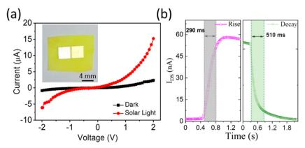
Fig. 4 (a) I-V curves of Au/MQDs@10/CNF/Pt under dark and solar light illumination. The inset shows the photograph of the Au/MQDs@10/CNF/Pt device. (b) Temporal photocurrent responses highlight a rise time of 290 ms and a decay time of 510 ms.
