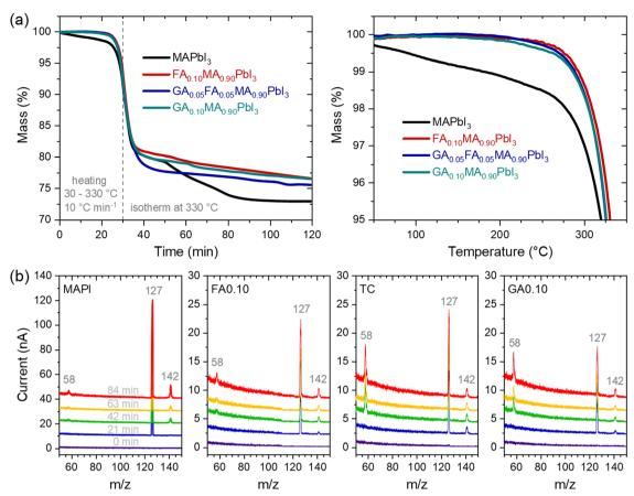
Fig. 4 (a) Mass percentage as a function of time (left) and temperature (right) under heating in two regimes. The figure on the right is a zoomed-n version for better visualization of the composition differences. (b) Cumulative mass spectra in the *m/z* range from 50 to 150 collected at different times under heating. Vertical shifts between the spectra were made intentionally for better visualization of the results.
