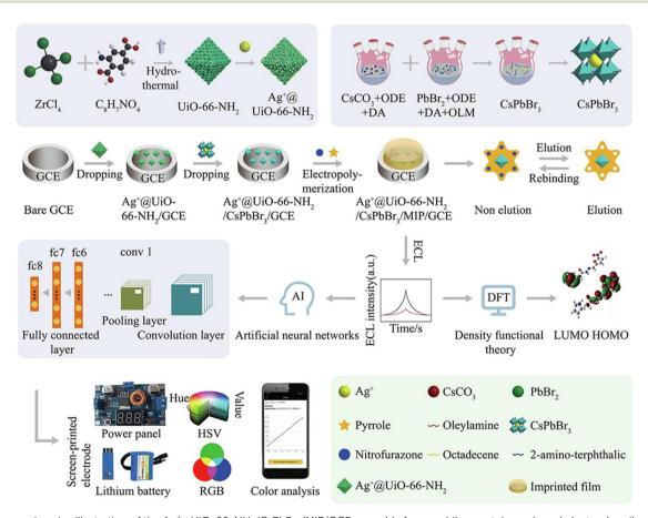
Fig. 4 A comprehensive illustration of the Ag+aUiO-66-NH<sub>2</sub>/CsPbBr<sub>3</sub>/MIP/GCE assembly for a mobile smartphone-based electrochemiluminescence molecularly imprinted polymer (ECL-MIP) system, depicting the intricate steps of preparation, integration of machine learning techniques, and the sensing mechanism. Adapted with permission. 123 Copyright 2022, Elsevier.
