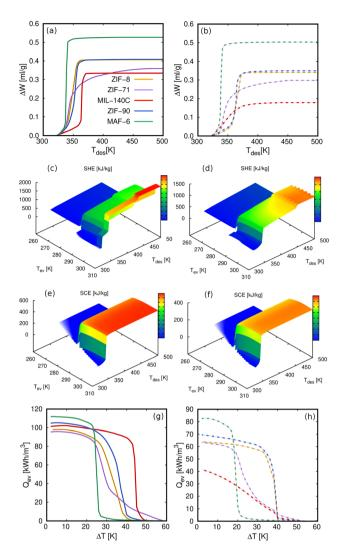
Fig. 12 Deliverable capacity for (a) methanol and (b) ethanol as a function of the desorption temperature for  $T_{\rm ev}=300$  K and  $T_{\rm con}=$ 310 K. The SHE and SCE of (c and e) methanol and (d and f) ethanol in MAF-6 at  $T_{con} = 313$  K.  $Q_{ev}$  as a function of temperature lift  $(T_{con} - T_{ev})$ , for (g) methanol and (h) ethanol varying  $T_{ev}$  with  $T_{con}$  and  $T_{des}$  set to 298 K and 373 K, respectively.
