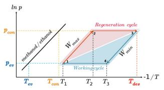
Fig. 1 Isosteric cycle of an AHP, including vapor pressure of alcohol molecules (black line), temperature and pressure of the evaporator  $(T_{\text{ev}}, p_{\text{ev}})$ , and the condenser  $(T_{\text{con}}, p_{\text{con}})$ , desorption temperature  $(T_{\text{des}})$ , and intermediate cycle temperatures  $(T_{(1-3)})$ . The working cycle (adsorption) is highlighted in blue and the regeneration cycle (desorption), in red.
