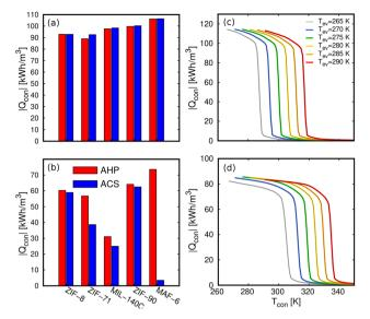
Fig. 11 Volumetric heat energy transferred to the condenser per unit of volume of the MOF using (a) methanol and (b) ethanol for the AHP (red) at  $T_{\rm ev} =$  273 K and  $T_{\rm con} =$  288 K and ACS (blue) at  $T_{\rm ev} =$  283 K and  $T_{con} = 298$  K. Volumetric heat energy transferred to the condenser per unit of volume of the MOF using (c) methanol and (d) ethanol in MAF-6 with variation of the temperature of the evaporator assuming full desorption
