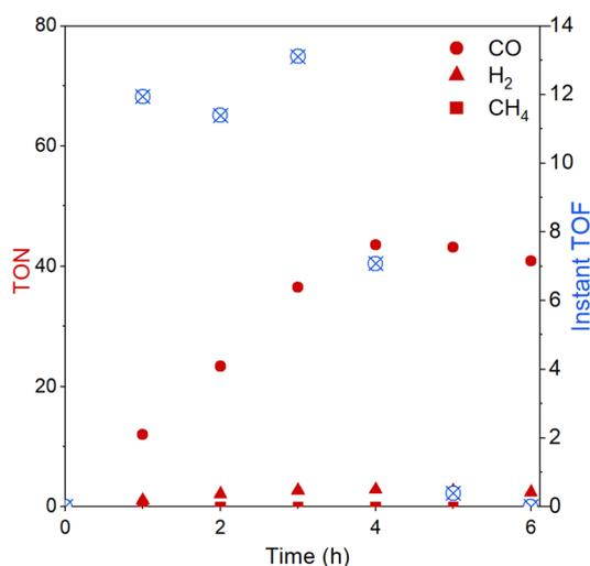
Fig. 5 Turnover number (TON) and instant turnover frequency (instant TOF) of CO<sub>2</sub> reduction reaction over the time course of 6 h with CLP-1.
