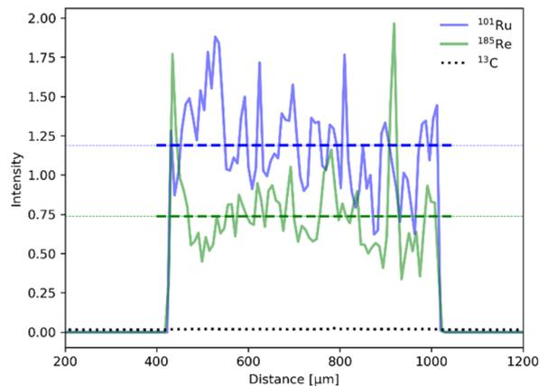
Fig. 4 LA-ICP-MS line scan for <sup>101</sup>Ru (red) and <sup>185</sup>Re (green) normalized to the <sup>13</sup>C isotope (black, dotted). Average intensity for each isotope is depicted as dotted line.
