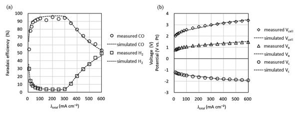
Fig. 7 CO<sub>2</sub> EC performance versus total current density ( $J_{\text{total}}$ ). (a) faradaic efficiencies of CO and H<sub>2</sub>. (b) Cell voltage ( $V_{\text{cell}}$ ), anode potential ( $V_{\text{a}}$ ), and cathode potential  $(V_c)$  (CO<sub>2</sub> flow rate, 5 sccm cm<sup>-2</sup>; cell temperature, 50 °C). Markers show measured values and dotted lines show simulated values.
