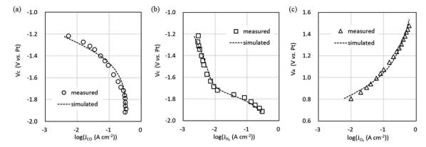
Fig. 6 Measured cathode potential  $V_c$  and anode potential  $V_a$  relative to the Pt pseudo-reference electrode and simulation using the equivalent circuit model in Fig. 2b. (a) CO evolution reaction (COER). (b) H<sub>2</sub> evolution reaction (HER). (c) O<sub>2</sub> evolution reaction (OER).
