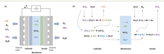
Fig. 1 Schematic drawing of (a) configuration of zero-gap type CO<sub>2</sub> EC producing CO and (b) electrochemical and chemical equilibrium reaction steps.
