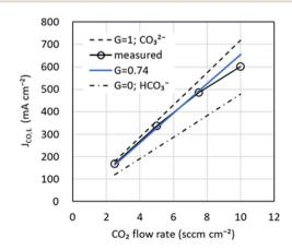
Fig. 4 CO limiting current density versus CO<sub>2</sub> flow rate input from the cathode channel. Markers are experimental values. Dotted, dotteddashed, and solid blue lines are calculated values for G = 1 (CO<sub>3</sub><sup>2-</sup>), G= 0 (HCO<sub>3</sub><sup>-</sup>), and G = 0.74 (CO<sub>3</sub><sup>2-</sup>; 74%, HCO<sub>3</sub><sup>-</sup>; 26%), respectively. Gis the fraction of  $CO_3^{2-}$  that transfers from the cathode to the anode.
