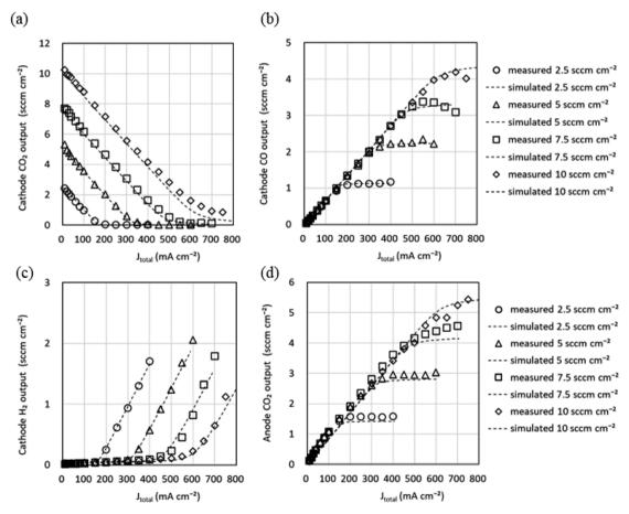
Fig. 8 Gas flow rate output from the cathode and anode channels *versus* total current density ( $J_{\text{total}}$ ) for four CO<sub>2</sub> input flow conditions. (a) CO<sub>2</sub>, (b) CO, and (c) H<sub>2</sub> are output from the cathode channel. (d) O<sub>2</sub> is output from the anode channel. Experimental data are shown as markers and simulation data using the values listed in Tables 2 and 3 and G = 0.74 as dotted lines.
