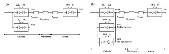
Fig. 2 Equivalent circuit models for  $CO_2$  EC. (a) Equivalent circuit of the cathode with a parallel connection between a COER element and one HER element. (b) Equivalent circuit of the cathode with a parallel connection between a COER element and two HER elements (low current density and high current density).
