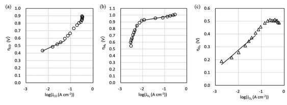
Fig. 5 Tafel plots at a CO<sub>2</sub> flow rate of 5 sccm cm<sup>-2</sup> and cell temperature of 50 °C. (a) CO evolution reaction (COER). (b) H<sub>2</sub> evolution reaction (HER). (c) O<sub>2</sub> evolution reaction (OER).
