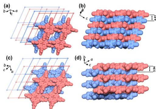
Fig. 7 The AA stacking pattern of HOF-29 viewed perpendicularly (a) and side views (b); the AB stacking pattern of HOF-29 viewed perpendicularly (c) and side views (d).<sup>57</sup>
