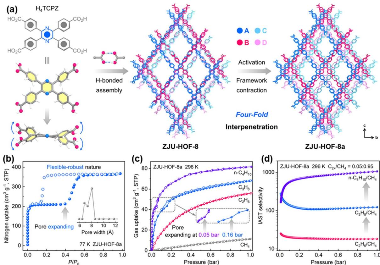
Fig. 13 (a) Single-crystal structure of ZJU-HOF-8 and the structural transformation with framework contraction upon activation; (b)  $N_2$  adsorption of ZJU-HOF-8a at 77 K; (c) different gas adsorption at 296 K; (d) IAST selectivities of ZJU-HOF-8a at 296 K.<sup>55</sup>
