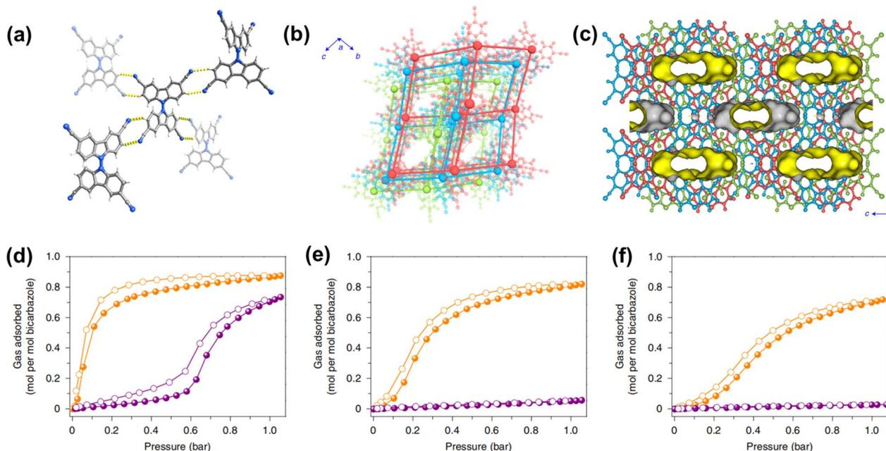
Fig. 6 (a) The intermolecular H-bonding interactions between bicarbazole units; (b) the threefold-interpenetrated dia net; (c) pore channels along the [100] direction; (d–f) gas adsorption isotherms for  $C_2H_4$  (orange) and  $C_2H_6$  (purple) at 298 K, 318 K and 333 K, respectively.<sup>52</sup>
