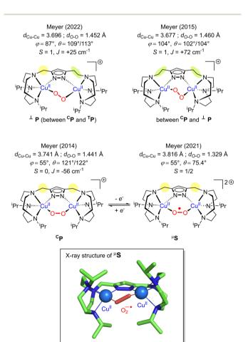
Fig. 8 Summary of the structurally characterized dicopper(II) peroxido species with pyrazolato/TACN based ligands from the Meyer group. ^160-162,167  $\varphi$  represents the torsion angle Cu-O-O-Cu and  $\theta$  the Cu-O-O angle
