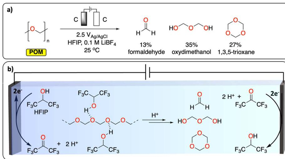
Fig. 3 Electrochemical depolymerization of POM. (a) Reaction conditions reported to generate formaldehyde, formic acid and 1,3,5-trioxane *via* electrochemical depolymerization of POM. (b) The dual role of HFIP in breaking the crystallinity of POM and in generating H<sup>+</sup> during its oxidation to trigger POM depolymerization.<sup>28</sup>
