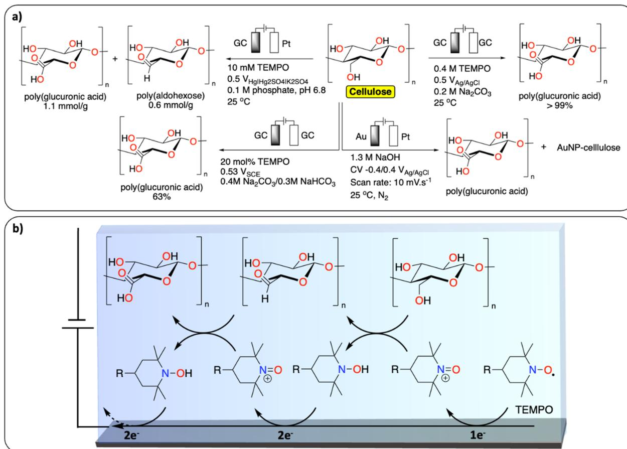
Fig. 8 Electrochemical PPF of cellulose. (a) Scheme of reaction conditions reported for the electrochemical PPF of cellulose;<sup>74–76,78</sup> (b) example of proposed mechanism of TEMPO mediated electrochemical oxidation of cellulose.
