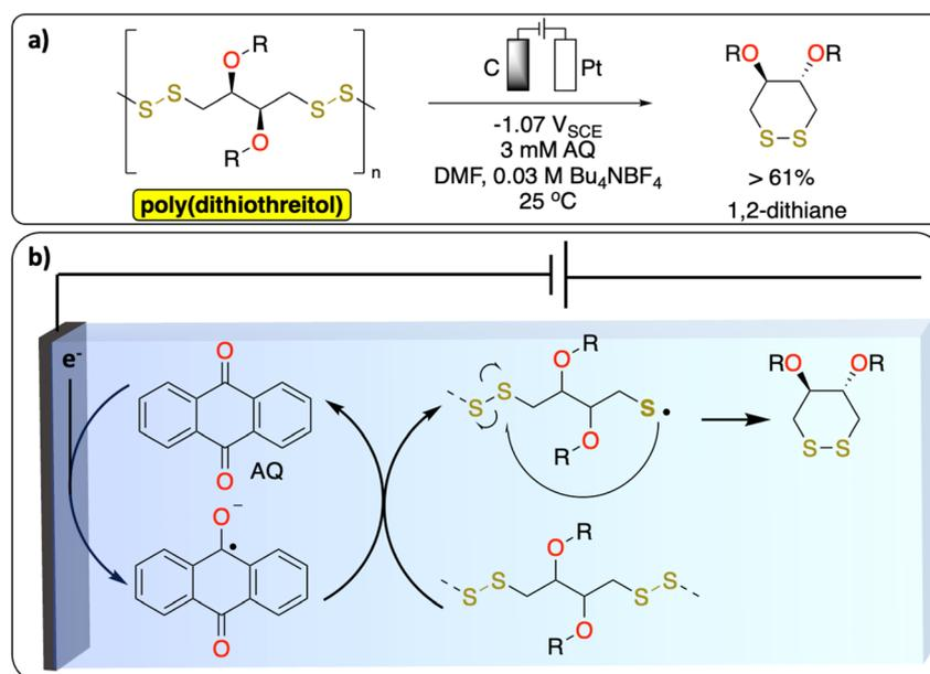
Fig. 5 Redox-mediated electrochemical depolymerization of poly(dithiothreitol). (a) Scheme of the reaction. (b) Proposed mechanism.<sup>54</sup>
