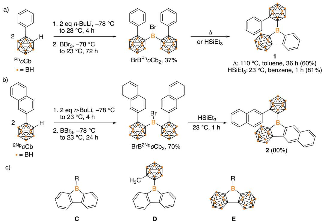
Fig. 2 Synthesis of hybrid carborane-arene borafluorenes **1** (a) and **2** (b), structures of borafluorenes **C** and **D**, 3D analogue **E** (c).
