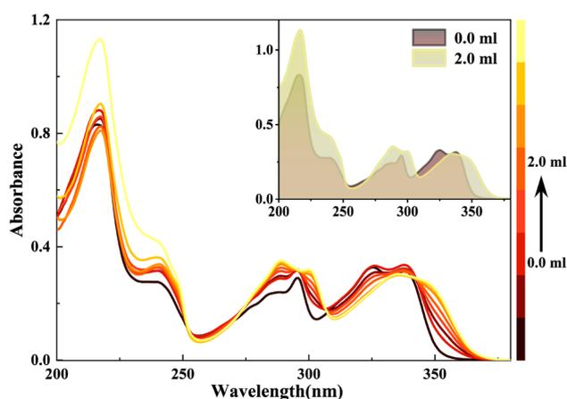
Fig. 5 UV-Vis spectra of a  $2.5 \times 10^{-5}$  M HBI-pBr solution in  $\text{CH}_3\text{OH}$  as a function of  $\text{CF}_3\text{COOH}$  (TFA,  $2.0 \times 10^{-4}$  M) in  $\text{CH}_3\text{OH}$  from 0 to 2.00 mL.
