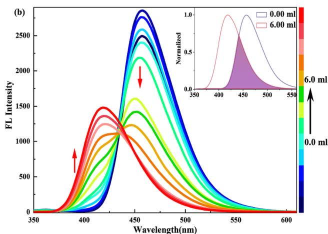
Fig. 4 (a) Excitation ( $\lambda_{em} = 419.0$  nm) and (b) emission spectra ( $\lambda_{ex} = 340.0$  nm) of  $2.5 \times 10^{-5}$  M HBI-pBr in  $\text{CH}_3\text{OH}$  as a function of  $2.0 \times 10^{-4}$  M  $[(\text{Bu})_4\text{N}]\text{OH}$  solution in  $\text{CH}_3\text{OH}$  from 0 to 6.00 mL.
