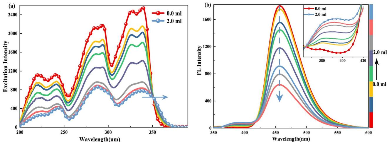
Fig. 6 (a) Excitation ( $\lambda_{em} = 391.0$  nm) and (b) emission spectrum ( $\lambda_{ex} = 340.0$  nm) of  $2.5 \times 10^{-5}$  M HBI-pBr in  $\text{CH}_3\text{OH}$  doped with different volumes of as a function of  $2.0 \times 10^{-4}$  TFA solution in  $\text{CH}_3\text{OH}$  from 0 to 2.00 mL. Note: Inset shows normalized fluorescence emission spectra from  $V_{\text{TFA}} = 0$  to 2.00 mL.
