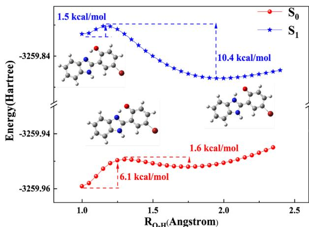
**Fig. 2** Potential energy curves for the S<sub>0</sub> and S<sub>1</sub> states of HBI-pBr calculated at the TD-B3LYP/6-311+G(d, p) level (step size 0.05 Å) using PCM (solvent = methanol) model.
