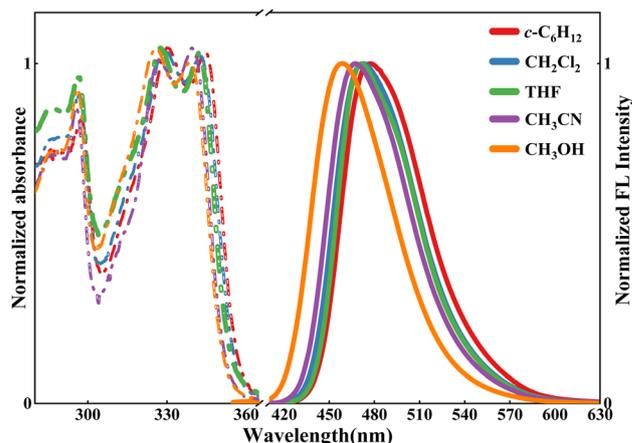
Fig. 1 Normalized absorption (dotted) and fluorescence spectra (solid,  $\lambda_{\text{ex}} = 340.0$  nm) in cyclohexane (c-C<sub>6</sub>H<sub>12</sub>), dichloromethane (CH<sub>2</sub>Cl<sub>2</sub>), tetrahydrofuran (THF), acetonitrile (CH<sub>3</sub>CN) and methanol (CH<sub>3</sub>OH).
