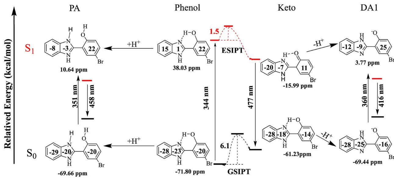
Fig. 7 Total and separately NICS(1)\_ZZ values (in ppm) of HBI-pBr and ions in the S<sub>0</sub> and S<sub>1</sub> states and the maximal absorption and emission bands observed experimentally.
