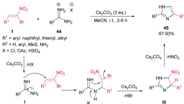
Scheme 21  $\text{Cs}_2\text{CO}_3$ -promoted reaction of bromonitroalkene with amidines.
