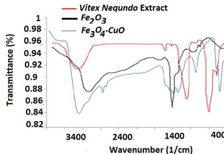
Fig. 2 FTIR spectrum of the VN-Fe<sub>3</sub>O<sub>4</sub>-CuO nanocatalyst.
