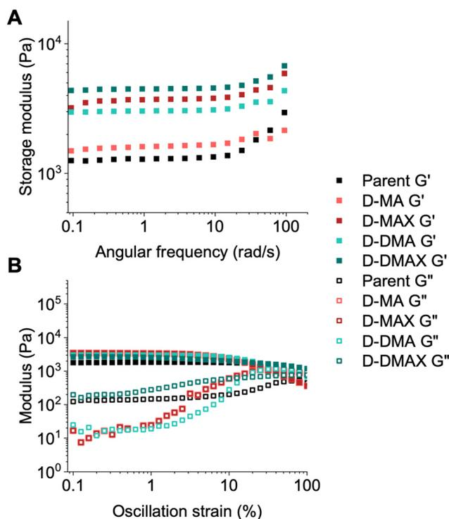
**Fig. 4** (A) Frequency sweeps of the parent and daughter gels. (B) Amplitude sweeps of the parent and daughter gels where the filled squares correspond to the storage modulus ( $G'$ ) and the empty squares correspond to the loss modulus ( $G''$ ).
