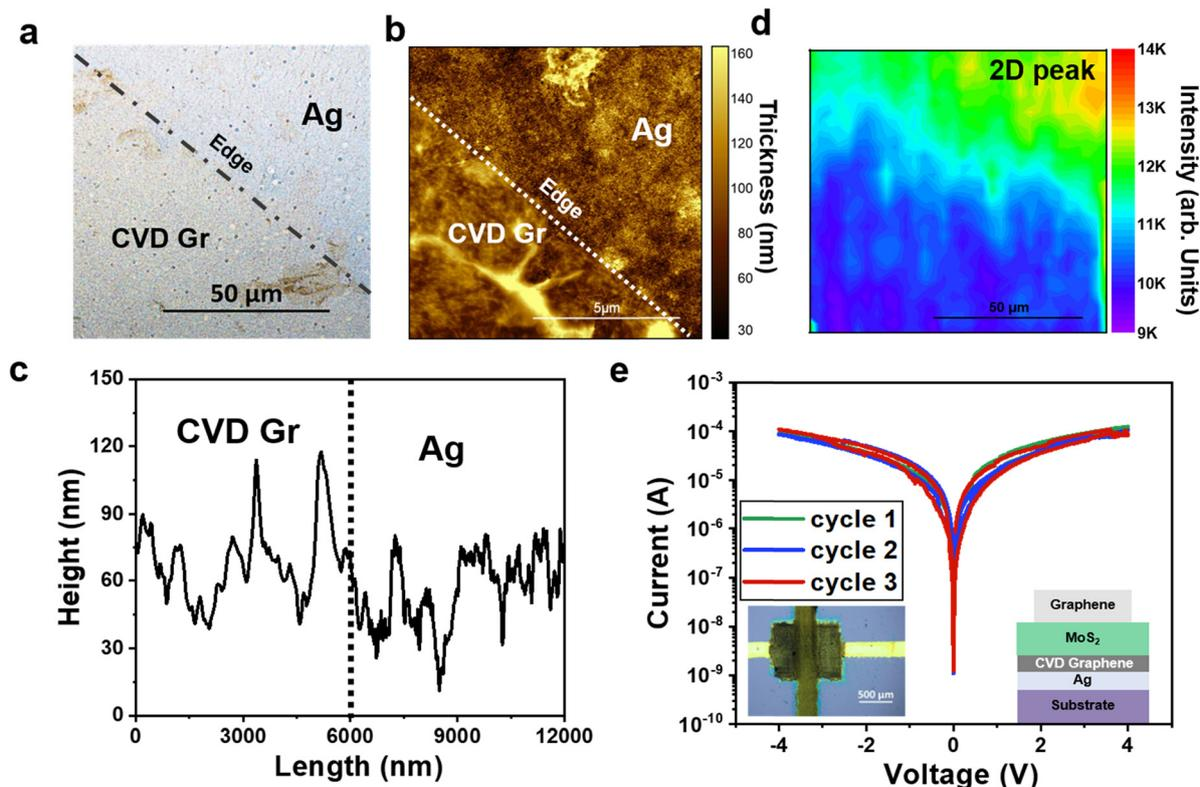
Fig. 4 Ag/MoS<sub>2</sub>/Gr memristors with integration of CVD graphene. (a) Optical image, (b) and (c) AFM image and (d) Raman mapping of the 2D peak intensity of CVD graphene transferred onto the printed Ag electrode. (e)  $I$ – $V$  curves of the Ag/CVD Gr/MoS<sub>2</sub>/Gr device; inset: optical image of the device.
