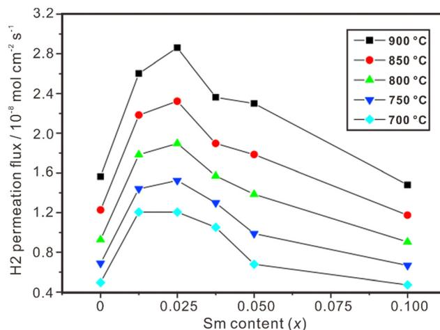
Fig. 11 Hydrogen permeation flux through  $\text{Ni}-(\text{La}_{1-x}\text{Sm}_x)_2\text{Ce}_2\text{O}_{7-\delta}$  membranes. Reprinted with permission,<sup>121</sup> Copyright [2010] Elsevier.
