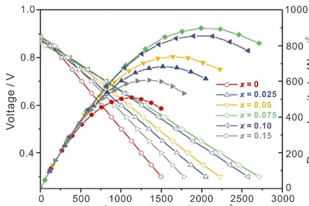
Fig. 10 Performance of fuel cells at 700 °C using  $(\text{La}_{1-x}\text{Mg}_x)_2\text{Ce}_2\text{O}_{7-\delta}$  as the electrolyte. Reprinted with permission,<sup>110</sup> Copyright [2019] Elsevier.
