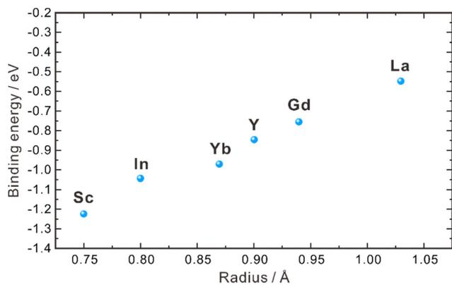
Fig. 2 Binding energies between dopants with different ionic radii and protons in the grain interior of  $\text{ZrO}_2$ .<sup>40</sup>
