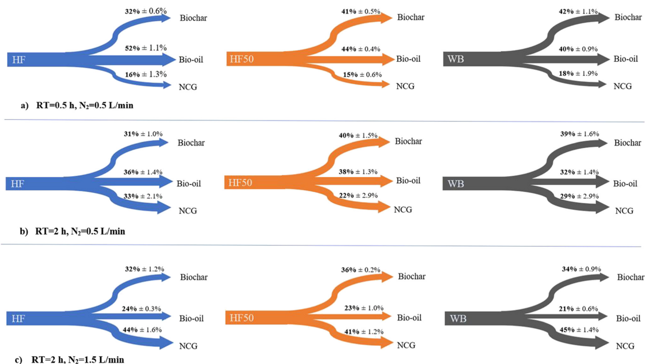
Fig. 8 Distribution of carbon flows to biochar, bio-oil and non-condensable gas (NCG) streams expressed as the % of the total carbon content in the feedstock (for HF, HF50 and WB) (pyrolysis experiments at 550 °C). Results for different combinations of retention time (RT) and N 2 gas flow rate: (a) RT = 0.5 h, N 2 = 0.5 L min -1 ; (b) RT = 2 h, N 2 = 0.5 L min -1 ; and (c) RT = 2 h, N 2 = 1.5 L min -1 . The reported values are calculated based on eqn (1)–(3), following total C analysis on a CHNS elemental analyser (see section 2.4).
