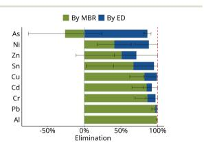
Fig. 5 Calculated elimination in the membrane bioreactor and retention in the electrodialysis of heavy metals and metalloids aggregated across phase I and phase II. The dashed line indicates 100% elimination.
