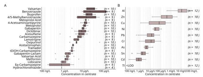
Fig. 2 Median concentration of organic micropollutants (A) and metals and metalloids (B) in the centrate used as feed for the nutrient recovery process aggregated over the study period. Samples were obtained directly prior to treatment in the MBR (n = n) number of detects in 10 (A) and 18 (B) samples). Concentrations distinguished for phases I and II are shown in Table S7.†
