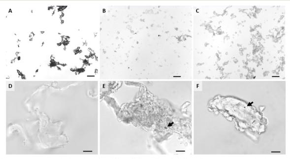
Fig. 1 Light micrographs showing abraded polymer (A and D) and 2% (B and E) and 0.5% (C and F) nanocomposite materials. Low magnification of materials are along the top row (A-C, scale bars 100 μm) and high magnification of each of those materials is along the bottom row (D-F, scale bars 20 µm). A and D) Abraded pristine PETG plastic; B and E) 2% AgNP nanocomposite; and C and F) 0.5% AgNP nanocomposite. Arrows point to AgNPs aggregates (dark dots) on or within PETG matrix.
